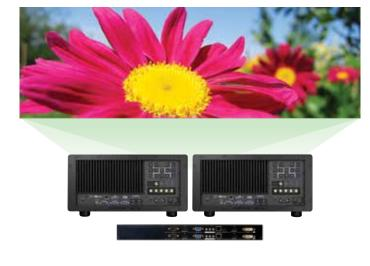
1 Use zoom and lens shift and focus to position the image of the projectors to cover the entire screen area
