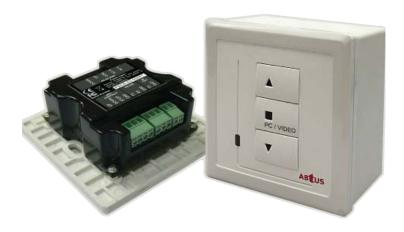
The ABtUS AVS-SSR8/1-1 is a Universal IR Motorized Screen and Projector Controller. It can easily be integrated into a Home Theater, Media Class Room, Meeting Room and more. It is also able to integrate with any third party central control system. Simple integration with direct power control of 220 to 240 VAC 50Hz/60Hz.
