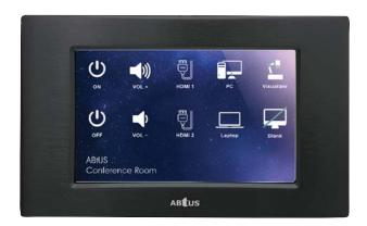
The ABtUS TP-05I is a TFT 65k true colour 5"LCD touch screen panel with a resolution of 800x480 pixels.
